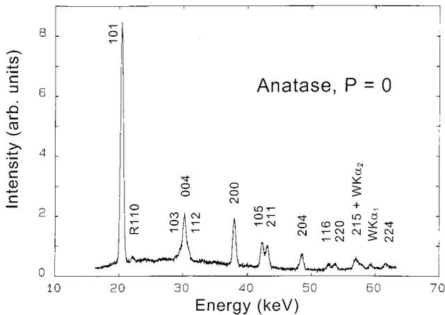
FIG. 1. Energy-dispersive powder-diffraction spectrum of TiO<sub>2</sub> at ambient pressure. Miller indices for the Bragg peaks are indicated. The Bragg angle is  $\theta=4.95^\circ$ . Intensities are given in arbitrary units. The peak denoted R110 is due to a small amount of rutile in the sample.
