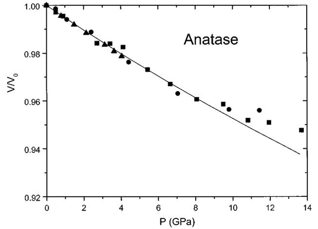
FIG. 4. Relative volume of anatase TiO<sub>2</sub>. Circles and squares denote two experimental runs with polycrystalline anatase, triangles denote single-crystal data, and the solid curve is the result of the theoretical calculation using the *ab initio* perturbed ion model.
