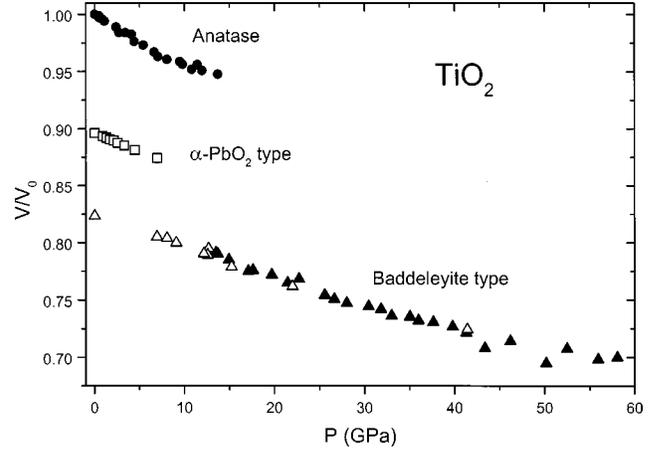
FIG. 3. Experimental pressure-volume data for the polycrystalline TiO<sub>2</sub> polymorphs investigated in the present work. The notation is the same as in Fig. 2. The unit-cell volumes have been normalized by dividing with  $V_{0,\text{anatase}}$ .
