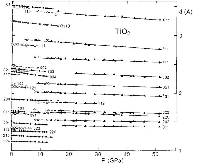
FIG. 2. Lattice plane spacing,  $d$ , obtained from powder diffraction, as a function of pressure,  $P$ . Circles denote anatase, triangles the baddeleyite phase, and squares the  $\alpha$ -PbO<sub>2</sub> phase. Filled symbols and full lines denote data obtained in a compression run, open symbols and broken lines denote decompression.
